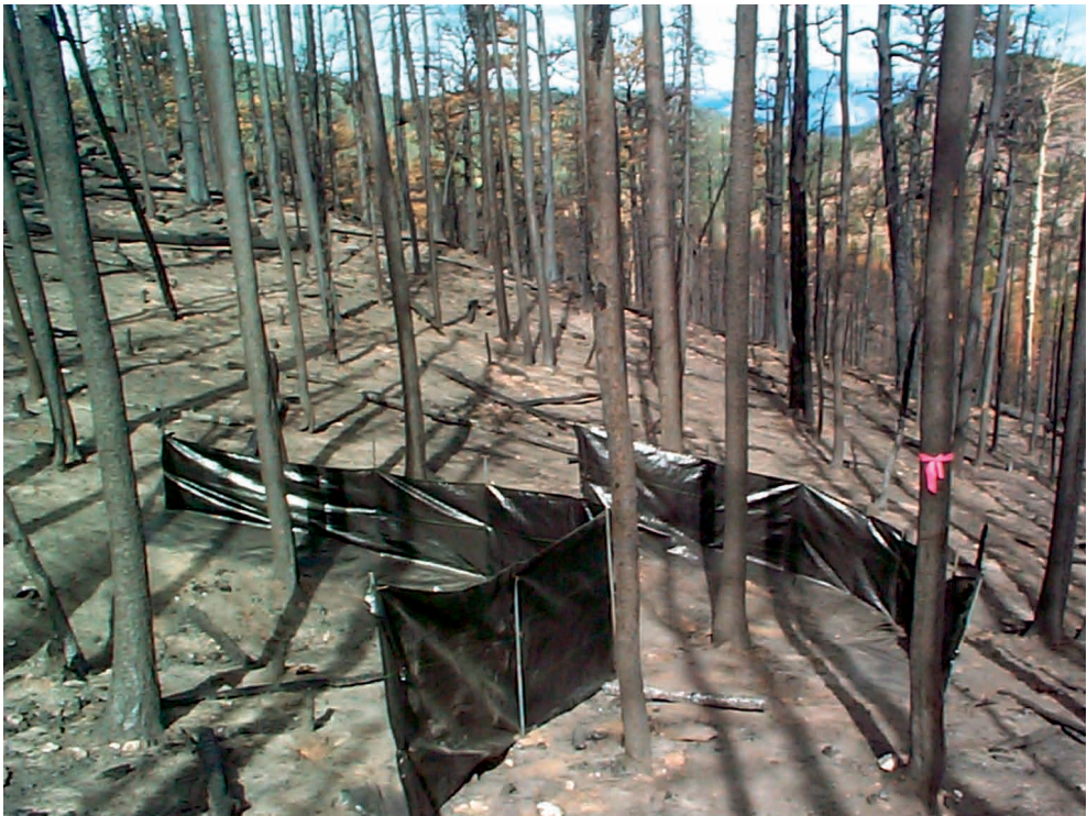
FIGURE 3. A pair of sediment fences used for measuring hillslope-scale sediment yields after a wildfire.
